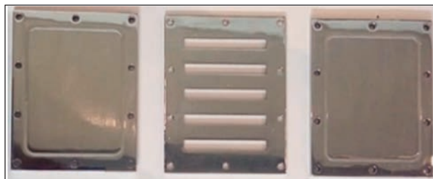
Figure-2: A three-piece stainless steel mould for impact strength.
